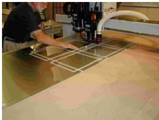
Grooving with CNC router
